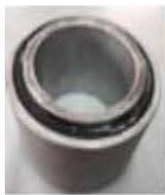
TRACTION CENTRE ELASTIC JOINT
