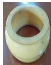
PAD FOR SECONDARY SUSPENSION
