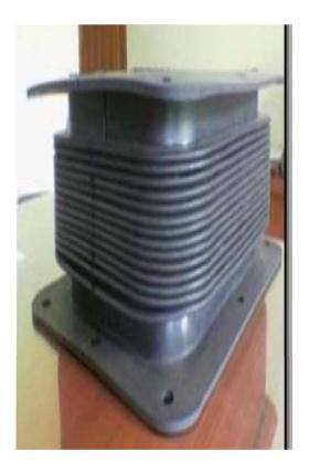
Standard size & weight: 445 mm x 342 mm Weight: 5 Kg. All Rubber Seamless One -Piece Moulded Traction Motor Bellow – Used as a type of exclusion seal to convey air from blowers inside the locomotive bodies to the commutated chamber of the traction motor
